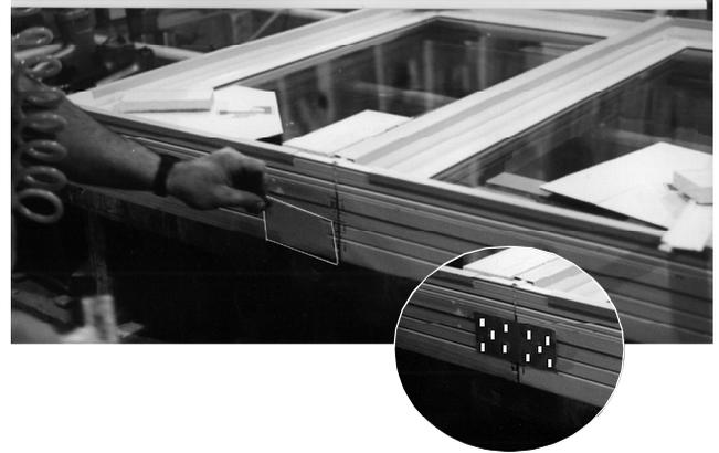
5. Using 1/2" x 3/4" staples, fasten structural mull plates to both the frame joints.
