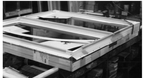
6. Apply the nailing fins, drip cap and corner protectors as required.
